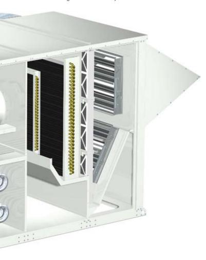
**AIR FILTRATION** 2, 4 or 6 inch pleated media filters are located in the mixed air chamber upstream of the cooling coil and are available with MERV ratings from 8 to 15.
