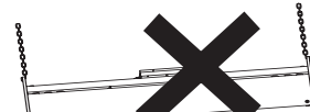
DO NOT Install So That Quartz Tube is Off Horizontal Like This
