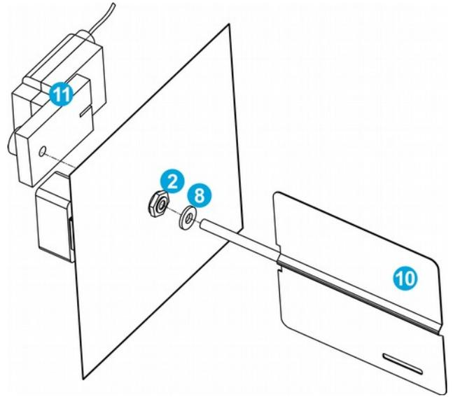
7. Expand the two blades to the maximum, then secure them in place by using loctite on both fixation studs and tightening the nuts.
