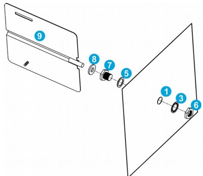
6. Insert a brass washer (8) on the driving blade shaft (10). Insert them through the through hole compression seal (2). Both blades should be resting on top of the other, with their threaded bolts inserted inside the appropriate openings.
