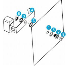
washer (3), the actuator mounting bracket (4), another lock washer (3), and a bolt (6). The actuator mounting bracket must either be perpendicular to the duct direction. Tighten fast.
